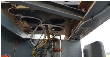
Strain gauges for WP unit force measurements
